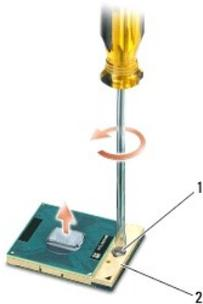
1 ZIF 插座凸面螺钉 2 ZIF 插槽
